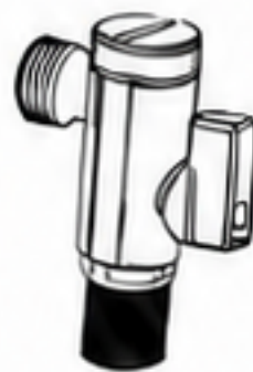
Integrated angle valve
